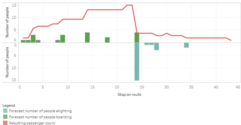
Figure 5.1: An example for the derivation of the number of passengers onboard from the forecasts of the two models.
